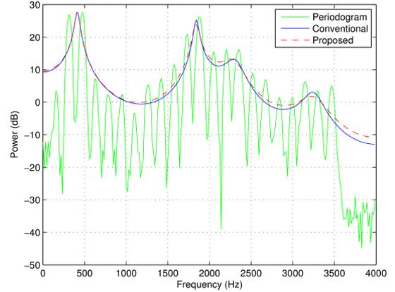
Figure 2: Periodogram  $P(k)$  with corresponding all-pole spectra of order  $p = 10$  computed by the conventional LP and the proposed BS-LP analysis method of clean speech (vowel /e/ produced by male speaker).
