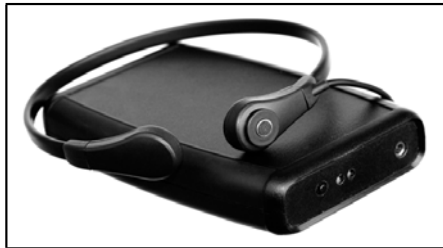
Figure 1: VoxLog lightweight portable voice accumulator.
